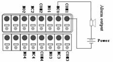
Fig 2.9 Alarm Output Connection
